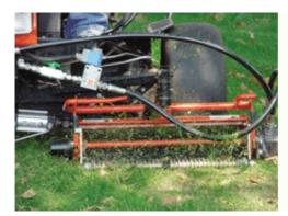
This industrial mower has been refitted with water hydraulics. The next test will use chrome-plated steel or plastic in place of aluminum.
